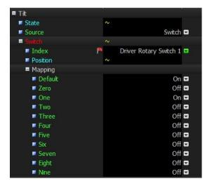
On the same worksheet, in the 'Main Switches' window, unassign the 'Resource' of the 'Driver Switch' that was initially used as 'Tilt Switch', this will be listed in the format 'CAN x Offset y'. Reassign this same resource to 'Driver Rotary Switch 1' in the same window. Set up the 'Driver Rotary Switch' as follows (note: this example uses 'CAN 2, Offset 0' as the resource):
